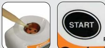
Fill the sample stage with the solution, put the metal anti-volatile cover on, and then press the START key.
