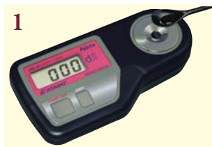
1 Apply 1 drop of sample solution onto the prism surface.
